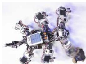
Following the principle of chaos control, the robot produces regular leg movements when walking normally. In addition, it can use the uncontrolled chaotic movement pattern to free itself when its leg is trapped in a hole.
