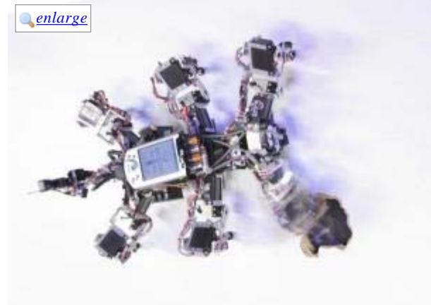
*Following the principle of chaos control, the robot produces regular leg movements when walking normally. In addition, it can use the uncontrolled chaotic movement pattern to free itself when its leg is trapped in a hole. (Credit: Network Dynamics Group, Max Planck Institute for Dynamics and Self-Organization)*
