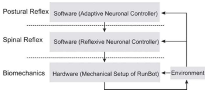
By dynamically adjusting posture and motor positions via input from sensors, the robot balances and adapts in realtime to terrain changes. A video of the robot walking, and adjusting its speed on the fly, can be seen [here](#) (MPEG). Very impressive how fast it walks (warms my heart).
