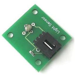
Sensor: A standard CdS (Cadmium Sulfide) photoresistor
