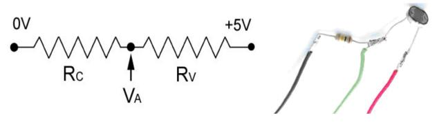
Here, our variable resistor is Rv and our constant resistor is Rc. Our measurement point 'A' is at the connection between the two resistors. Again let's start with the Ohm's Law:
