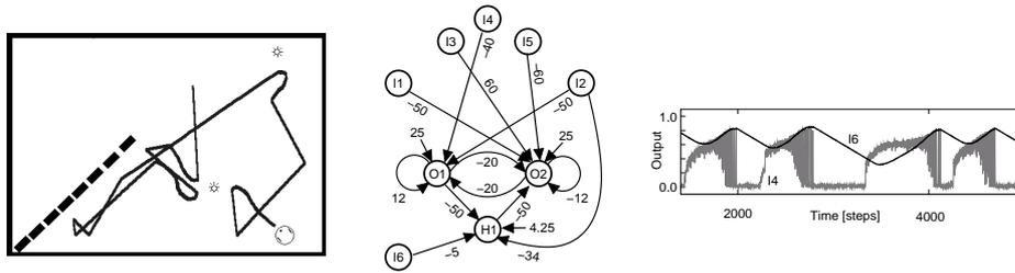
**Fig. 5.** The recurrent neural network producing a motivational driven robot behavior and the resulting behavior in simulation. The diagram shows the level of energy ( $I6$ , black) and activation of the frontal light sensor ( $I4$ , grey) during the interaction ( $f(x) = \sigma(x) = 1/(1 + e^{-x})$ ).
