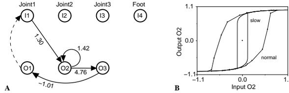
**Fig. 3.** A: Neural single-leg controller ( $f(x) = \tanh(x)$ ). B: Hysteresis of neuron  $O2$  (see text for details).
