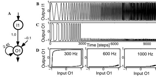
**Fig. 4.** A: A RNN ( $f(x) = \tanh(x)$ ) realizing low-pass filtering at  $\approx 300$  Hz. B,C: Input signal at increasing frequency (from 100 Hz to 1 kHz, 48 kHz sampling rate) and the corresponding output signal. D: The hysteresis effects between input and output signals at certain frequencies.
