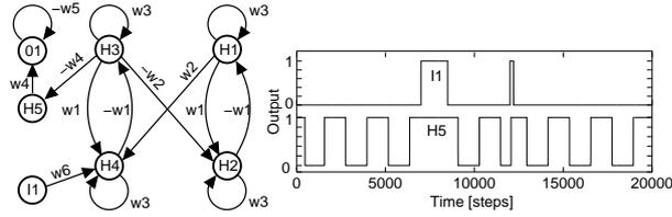
**Fig. 6.** An internal rhythm generator ( $f(x) = \sigma(x) = 1/(1 + e^{-x})$ ), and how it can be influenced by sensory stimuli.
