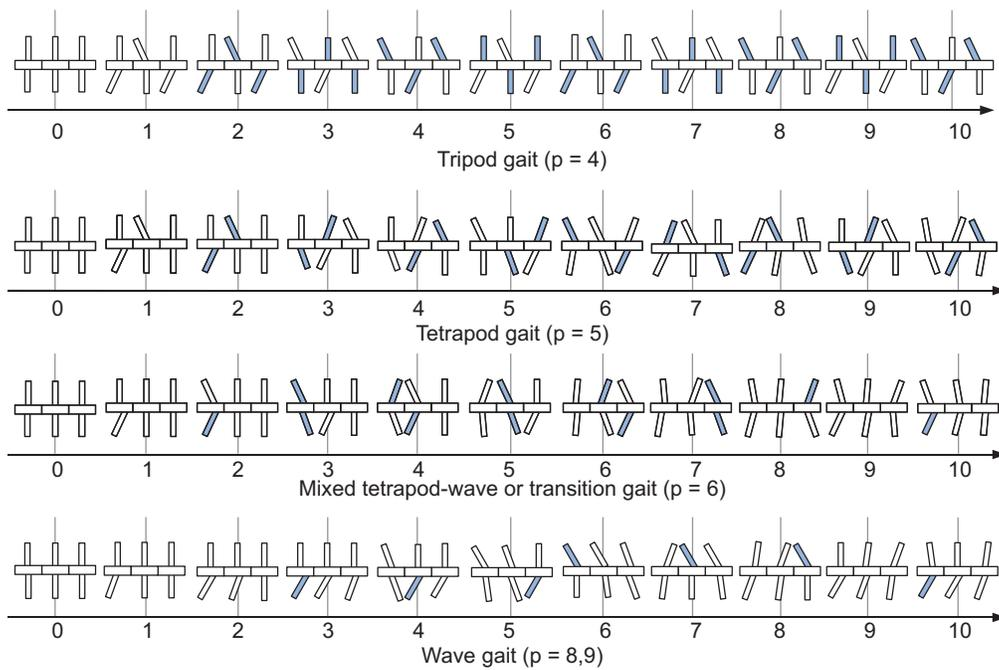
Supplementary Figure 4: **Sketch of different walking patterns according to target periods  $p$ .** A blue colored leg is in the air, a white leg is on the ground. To keep the images concise, only very coarse schemes are shown that do not take into account the different timings of swing and stance phases.
