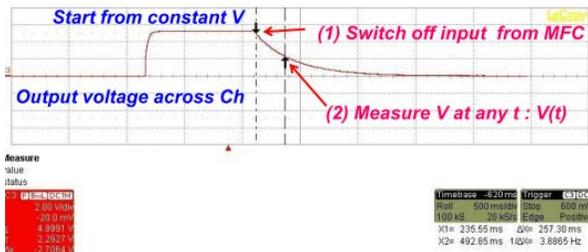
Fig. 4 Output voltage across capacitor in energy harvesting circuit for measuring internal resistance value.
