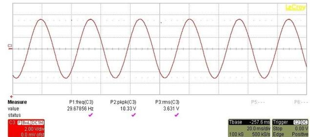
Fig. 7 Measured waveform of output voltage of MFC
