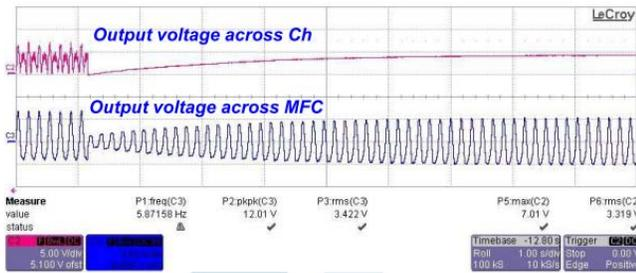
Fig. 3 Output voltage across MFC and capacitor in energy harvesting circuit.
