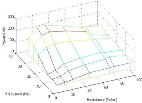
Fig. 9 Relation between  $R_{L\_peak}$ , frequency and harvested power (experimental results)
