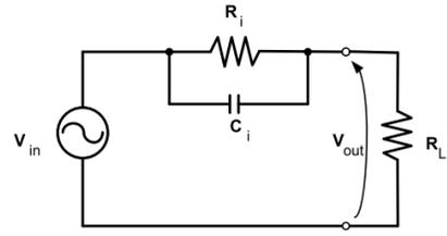
Fig. 1 Equivalent circuit of MFC
