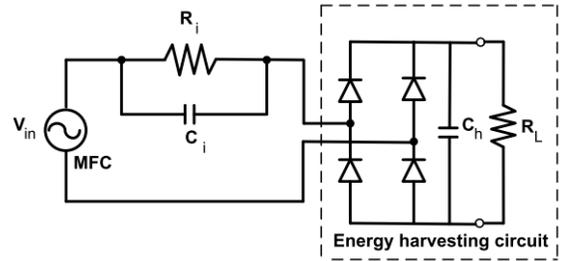
Fig. 2 Conventional energy harvesting circuit
