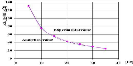
Fig. 8 Relation between  $R_{L\_peak}$  and frequency (simulated and experimental results comparison)
