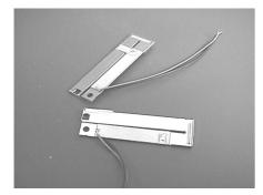
Figure 1: Piezoelectric PZT
