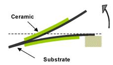
Figure 2: Diagram of the PZT piezoelectric
