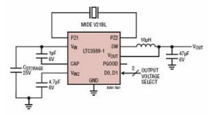
Figure 5: MFC Energy harvesting circuit diagram
