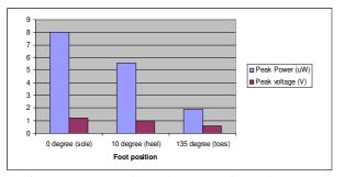
Figure 12: Peak voltage and peak power at prosthesis foot positions
