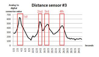
Fig. 11. Sensor output while roaming in an L-shaped environment
