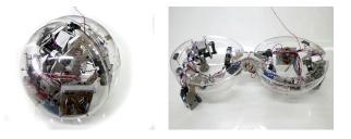
Fig. 1. A Reconfigurable Spherical Robot
