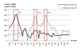
Fig. 15. Sensor output while roaming in a narrowing pathway
