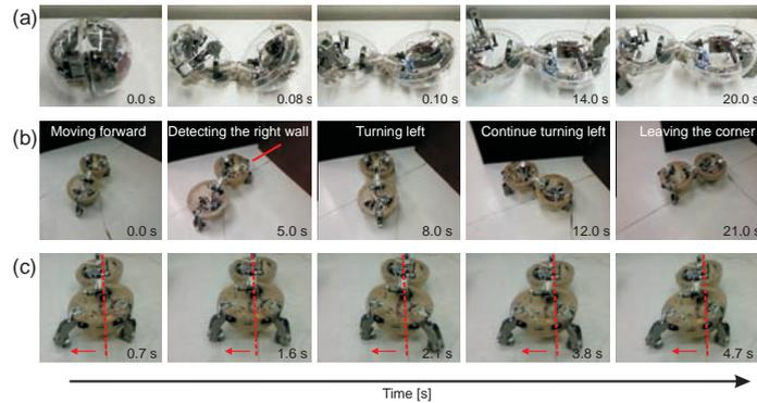
Fig. 4. (a) Transformation from the dormant mode to the transformed mode. (b) Obstacle avoidance behavior using wheels. (c) Sidestepping to the right using legs. The video clip of the tests including passive rolling motion can be see at <http://www.manoonpong.com/CLAWAR2013/S2.wmv>.
