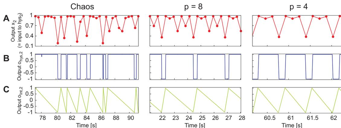
Supplementary Figure 3: **Postprocessing signals for different periods.** (A) Output signals of the time window function unit  $\Delta t$ . (B) Output signals of the hysteresis unit  $hys2$ . (C) Output signals of the signal integrator unit  $Int2$ .
