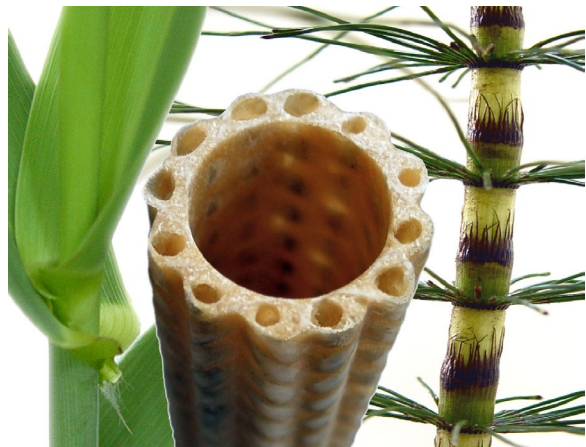
Fig. 3: The Technical Plant Stem (center) an ultra-lightweight fibrous compound structure with two of its biological models giant reed (left) and horsetail (right) © PBG Freiburg & ITV Denkendorf
