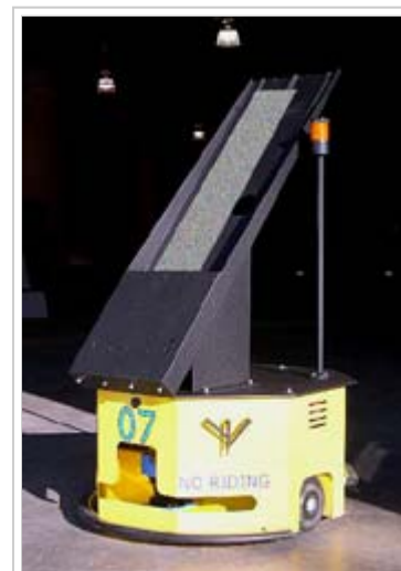
ADAM carries steel samples in a factory without following lines or triangulating from beacons.
