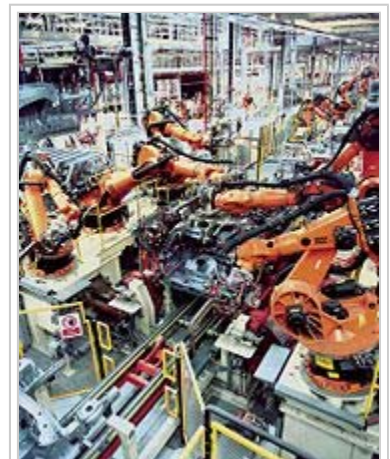
German KUKA Industrial robots doing vehicle under body assembly
